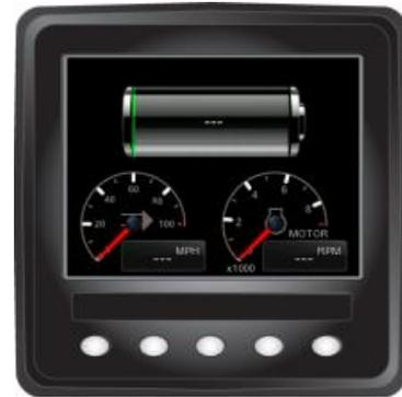
A custom Raptor screen showing a battery meter, vehicle speed and engine speed
