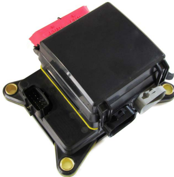
Figure 1. Multiplexed Vehicle Electrical Center
