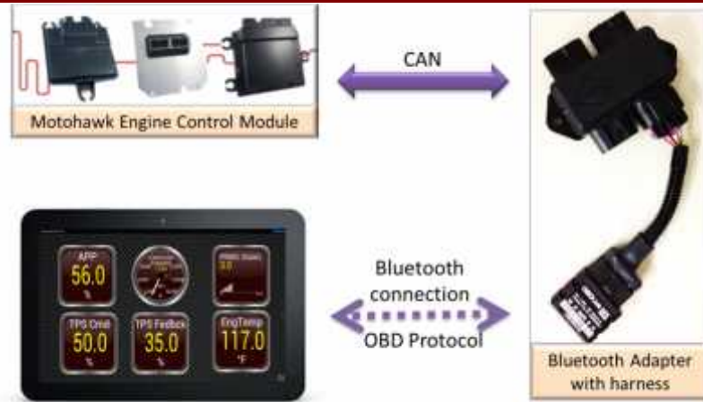
Figure 2 – The OBDII Bluetooth-CAN hardware connection
